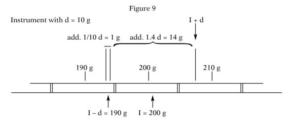
The indication at the start is I=200~g. Remove additional weights until the indication changes to I-d=190~g. Add 1/10~d=1~g and thereafter 1.4 d = 14 g. The indication shall then be I+d=210~g.
